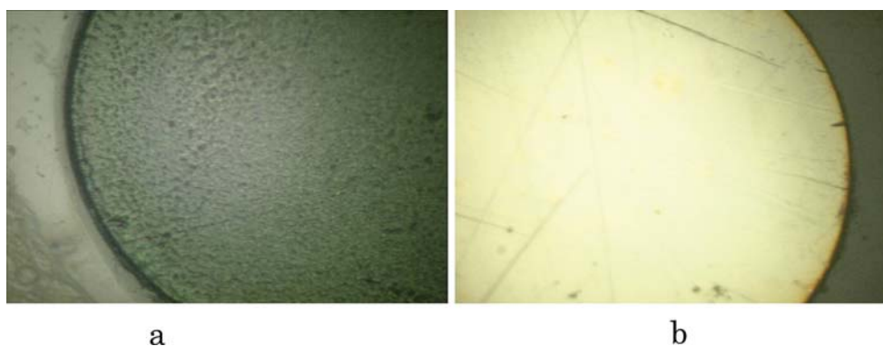
Fig. 4 Photographs of electro-polymerized film of PAB (a) and the bare Pt electrode 1.6 mm in diameter (b), obtained by the optical microscope
